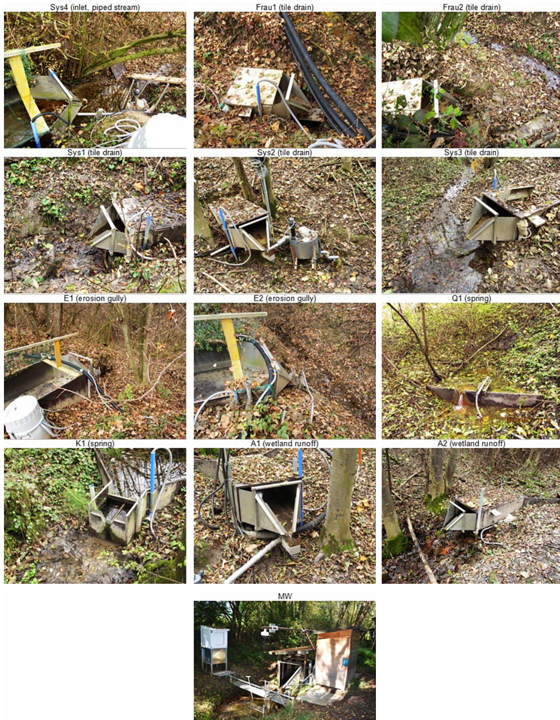
Figure C1. Photos of the 13 stream gauges in the HOAL.
