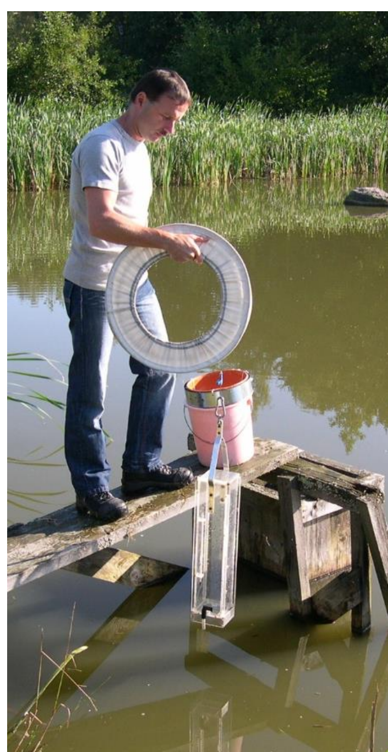
Fig. 1: Usage of a Schindler-Sampler, four samples on different places in the pond are taken for SV © BAW-ÖKO
