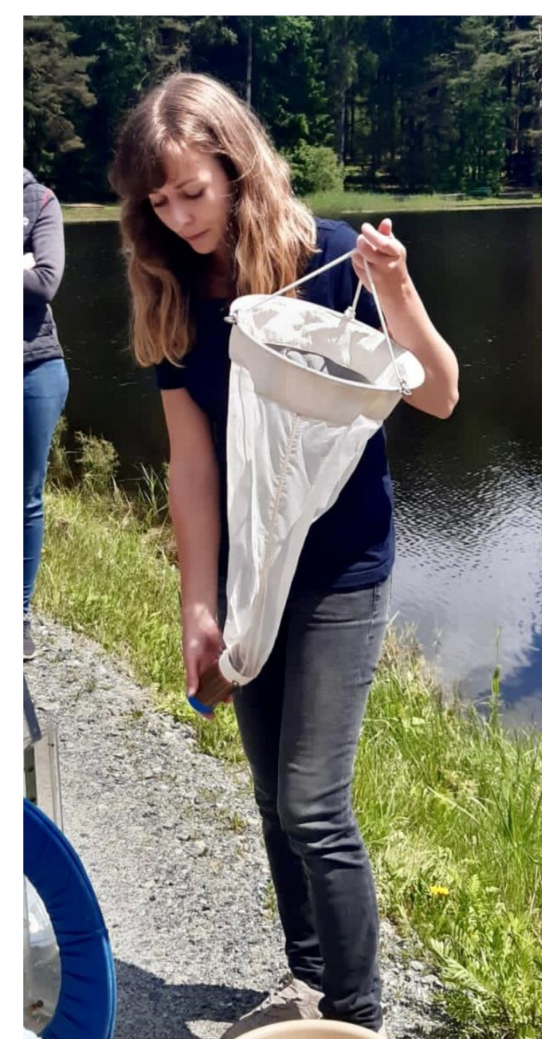
Fig. 2: The plankton net has a 500 µm patch on the cod end. © BAW-ÖKO
